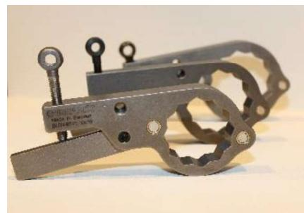
2. Choose an appropriate point of reaction. The BUW is intended to react firmly against an adjacent nut/screw head or solid reaction area in the same plane.
