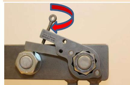
6. Use a suitable torque wrench to apply torque on the bolts to be tightened / off. Keep away from the BUW during operation and do not try to support it with your hands.
