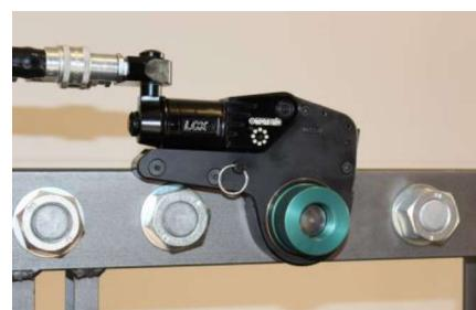
7. Once you tightened or loosened the screw you then turn the adjustment screw counter clockwise to unlock BUW from application. Make sure you hold the BUW to prevent it from falling down when loosened.
